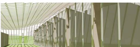
The screen has another function in that within the screen is running water being solar heated and pumped through the columns to be dispersed through a radiant heating and cooling system within the floor. The water can then be recycled back either through to the screen or to the actual roof creating a heat blanket and melting any snow fall in the winter.
