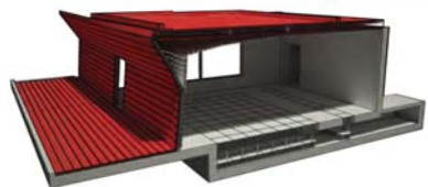
exterior wood skin and roofing structure
